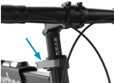
Stack Height Adjustment
